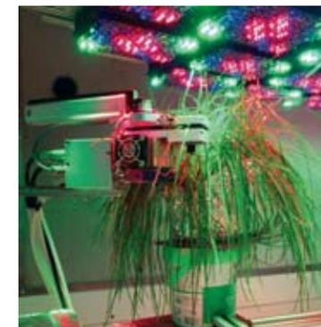
Artificial lighting provided by LED panel allows detailed manipulation of light quantity and quality
